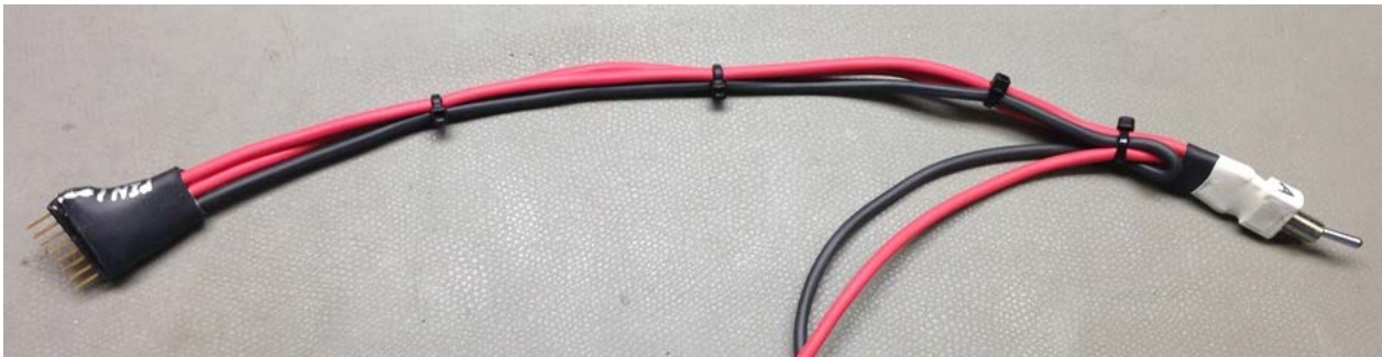
Plate 5 – Completed Calibration Harness
