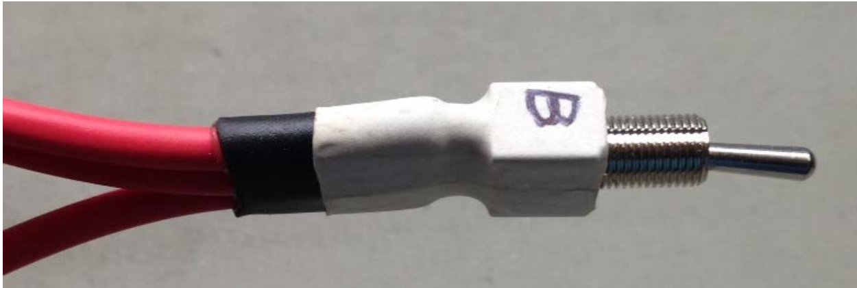
Plate 2 – Adhesive Lined Heat Shrink Tubing over Terminals with Label on Switch Housing
