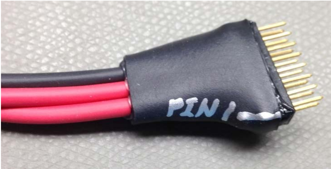
Plate 4 – Heat Shrink over Solder Joint
