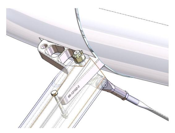
The above image shows a 66-12102-3 fitting with the engraved number on the aft-lower arm of the fitting. (FWD strut is transparent; view is aft-quartering, LHS, looking forward and inboard) (Note that the "-2" fitting is similar, but lacking the engraved number.)
