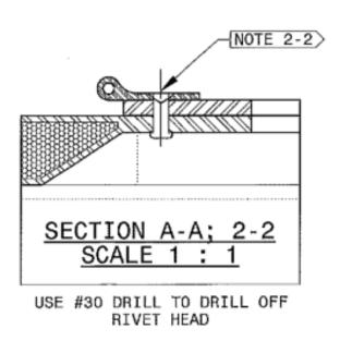
**CAUTION**: Avoid drilling too deeply as this may cause unnecessary damage to the door.
