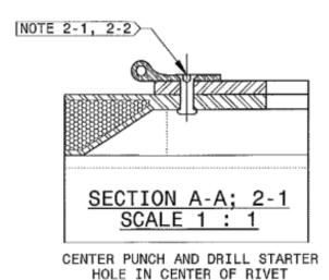
2.2 Pilot drill rivet heads with #50 drill, then drill #30 (Ø.1285) just to a depth that will allow it to be removed with a blunt punch. (Typically, (Ø.125" is inserted into the #30 hole, and pried side to side to remove the head.) The illustration below shows hull side hinge half. See Drawing 56-10113-SUPP Sheet 2.
