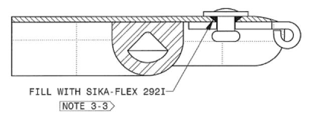
3.4 Install MS16353 rivets with NAS1149CN416R washers beneath heads.
