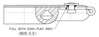
3.4 Install MS16535 rivets with NAS1149CN432R washers.
