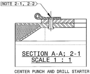
HOLE IN CENTER OF RIVET
