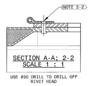
**CAUTION**: Avoid drilling too deeply as this may cause unnecessary damage to the door.
