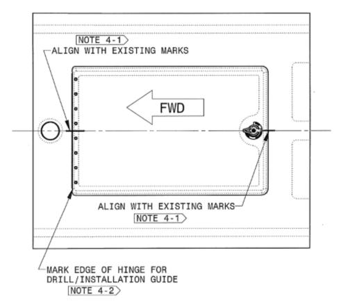
4.2 Mark the location of either the inboard or outboard edges of the hinge with a fine, felt-tipped pen.
