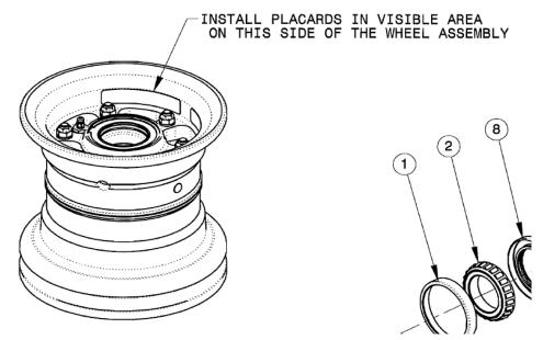
**Fig. 3** – 35A-51800 5.00 X 6.00 (6.00-6) Wheel Assembly, Oil Bath Type.
