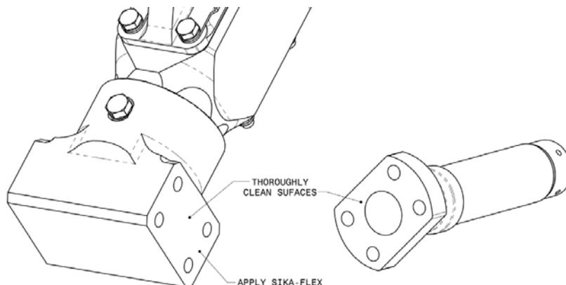
Cover this and opposite surface with sufficient amount of Sika-Flex 292 or similar marine grade adhesive to insure squeeze out at seams when bolted together.
