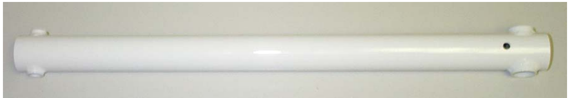
35-32155 nose drag brace after painting
