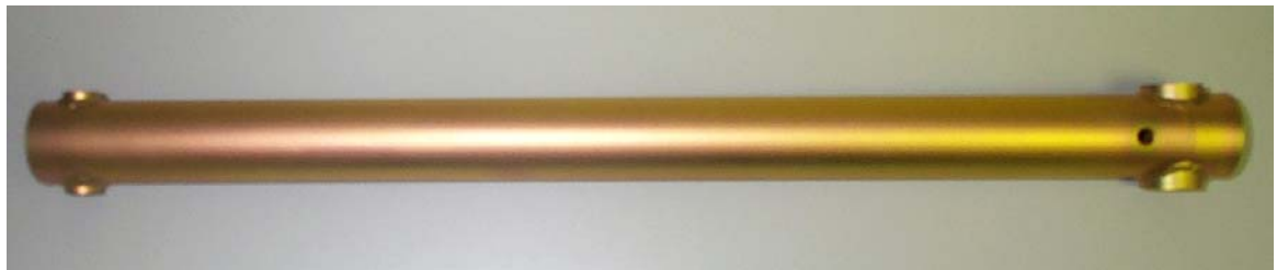
35-32155 cadmium plated nose drag brace before painting
