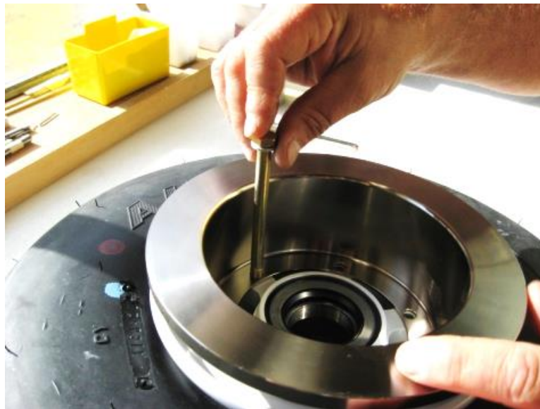
FIGURE 32-40-10-03-f Install tie bolts with washers from brake disc side of wheel assembly
