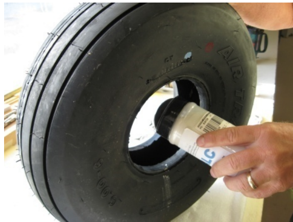
FIGURE 32-40-10-03-a Talcum powder aids in seating the inner tube
