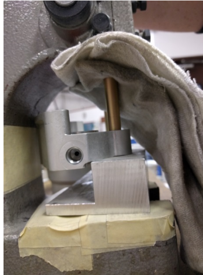
FIGURE 32-40-10-04-e Pressing anchor pin into brake housing with mechanical press.
