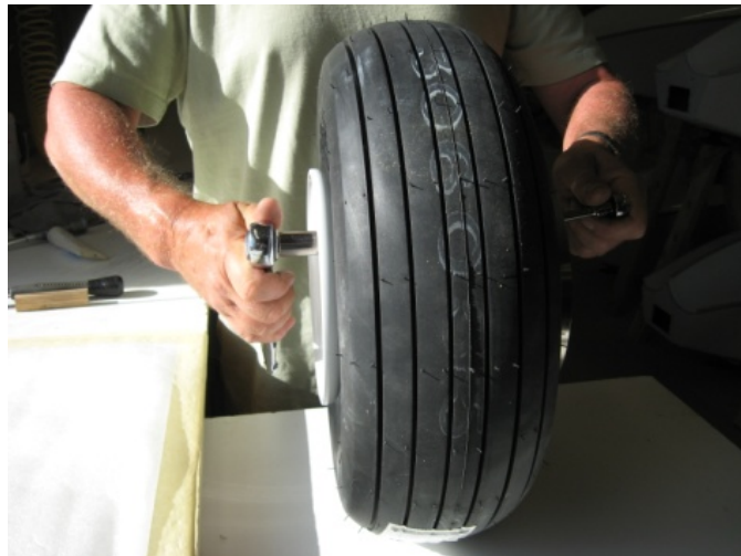
FIGURE 32-40-10-03-h Tighten nuts and tie bolts evenly with a diagonal crossing pattern
