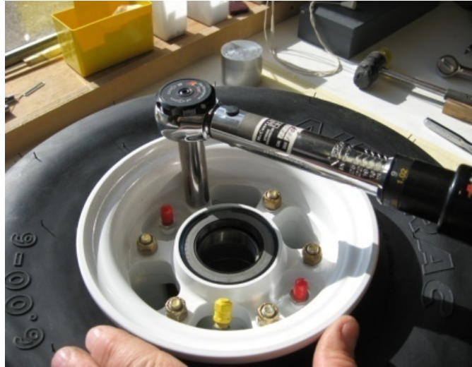
FIGURE 32-40-10-03-i Finish tightening nuts with torque wrench to values shown below.
