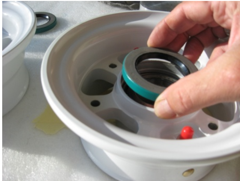
FIGURE 32-40-10-02-b Locate grease seal for press fit
