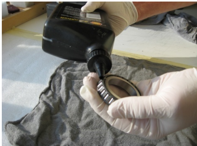
FIGURE 32-40-10-02-a Apply oil protection if wheel is to be stored before final assembly on aircraft
