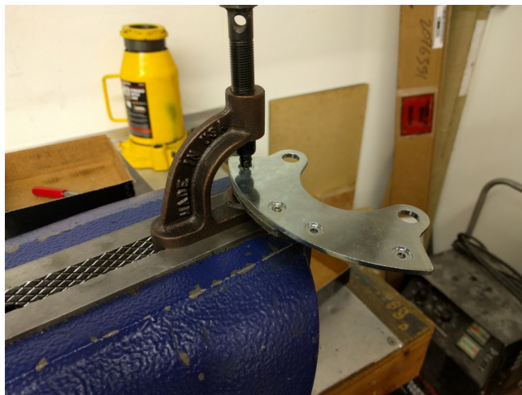
FIGURE 32-40-10-04-b Riveting Brake lining to pressure plate.
