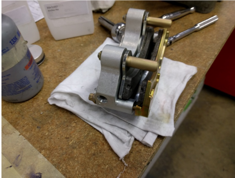
FIGURE 32-40-10-04-g Installing pressure and back plate to the brake housing.
