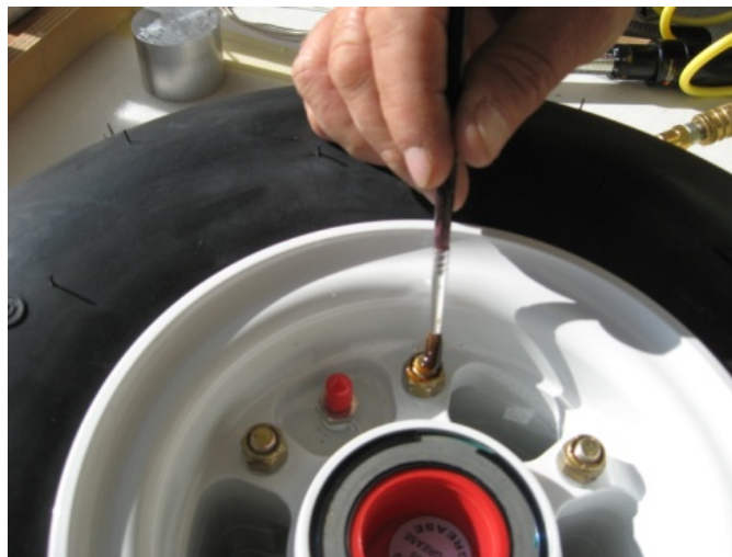
FIGURE 32-40-10-03-j Apply bolt protection to all exposed nuts, threads, bolt heads and fittings
