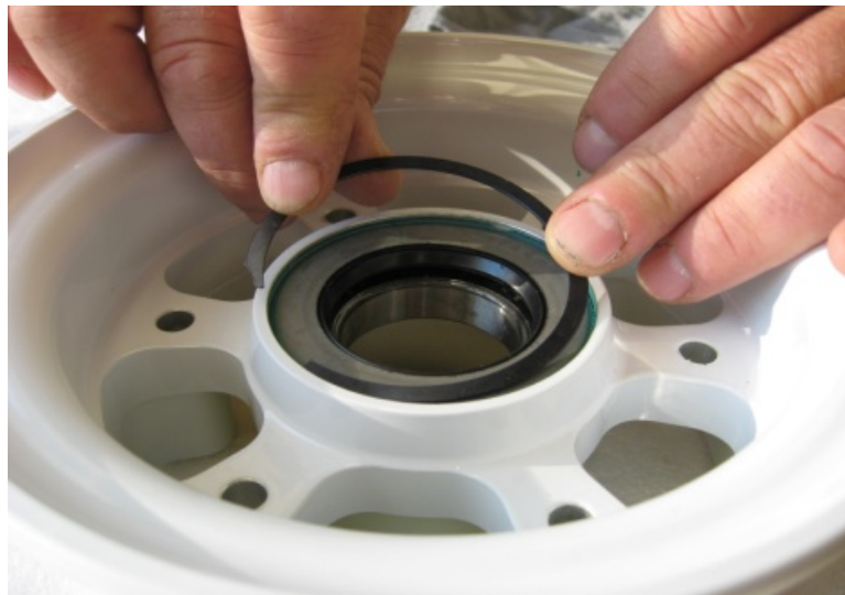
FIGURE 32-40-10-02-e Installing retaining ring
