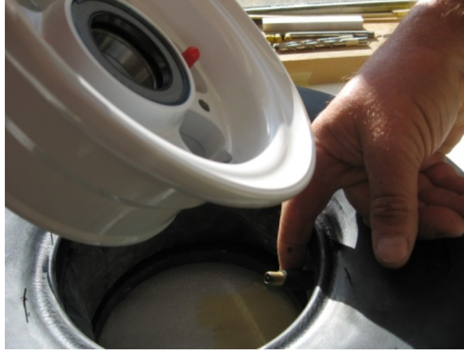
FIGURE 32-40-10-03-c Feed valve stem through port in hub and seat wheel half in tire
