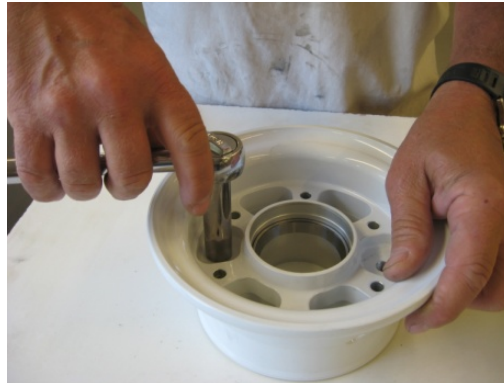
FIGURE 32-40-10-01-d Tighten brake bleeder assemblies, 2 locations on wheel half B
