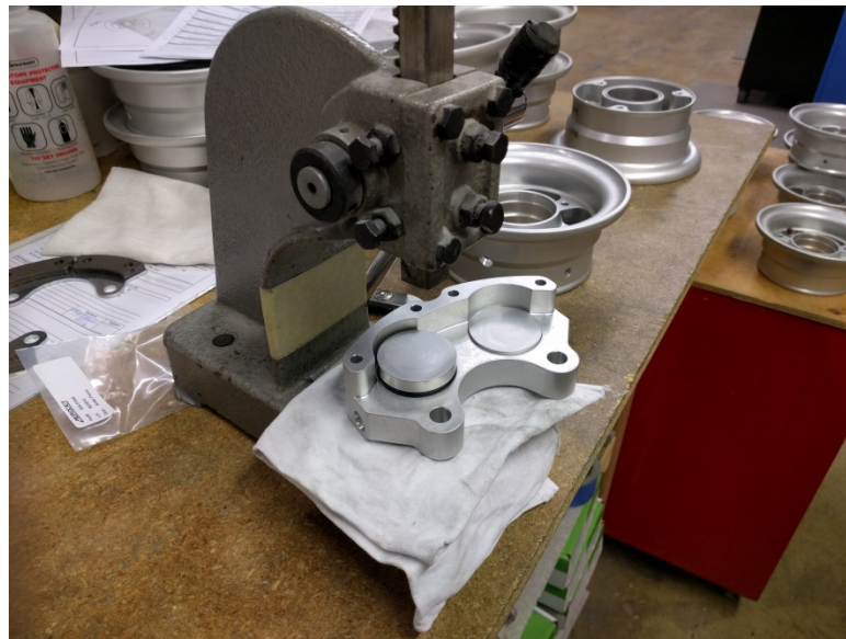
FIGURE 32-40-10-04-d Pressing brake pistons into brake housing with mechanical press.
