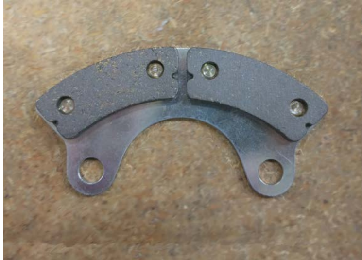
FIGURE 32-40-10-04-a Brake Lining rivet head orientation.
