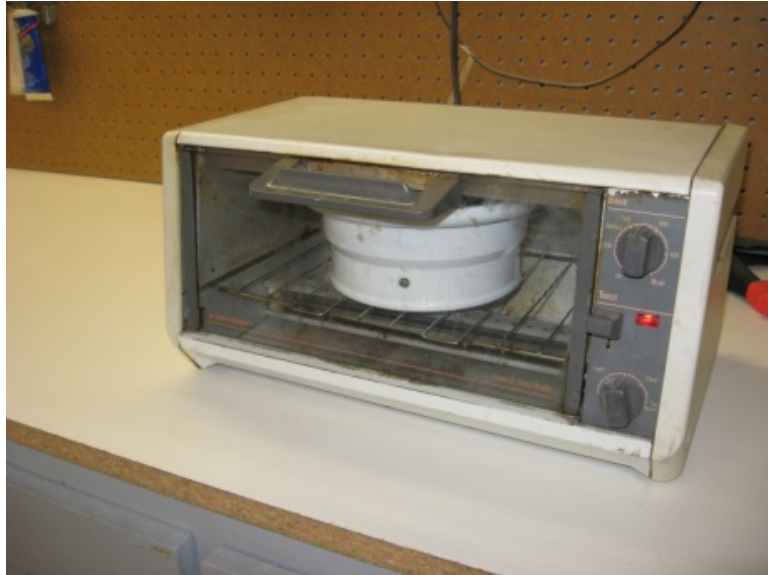
FIGURE 32-40-10-01-a Preheating wheel half in portable oven
