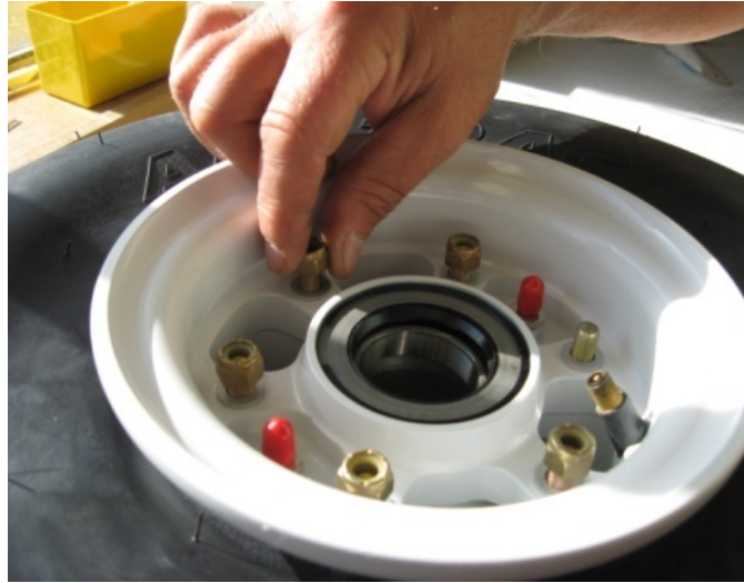
FIGURE 32-40-10-03-g Install self-locking nuts with washers
