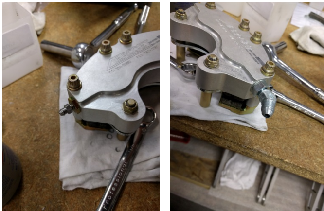
FIGURE 32-40-10-04-h Fitting Installed on Brake assembly.
