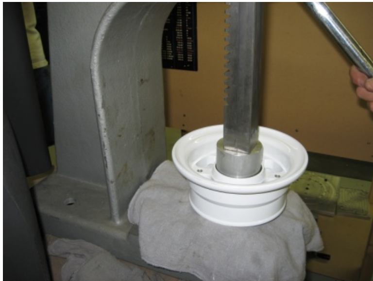
FIGURE 32-40-10-01-b Press fitting bearing cup with Arbor press
