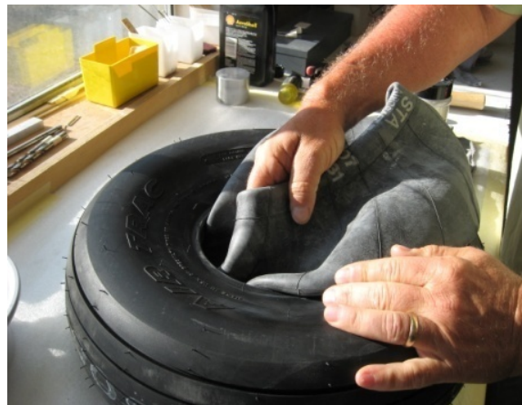
FIGURE 32-40-10-03-b Position tube loosely in tire
