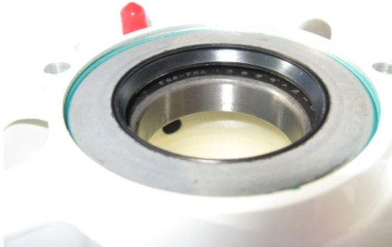
FIGURE 32-40-10-02-d Verify even access to the retaining ring groove. Seal must be flat, evenly installed to function properly. If the seal is incorrectly installed or damaged, then replace it.
