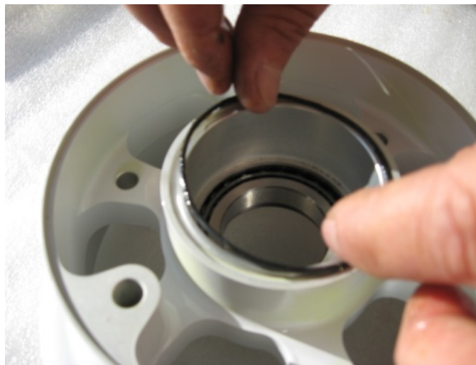
FIGURE 32-40-10-03-d Lithium grease holds o-ring in place during assembly
