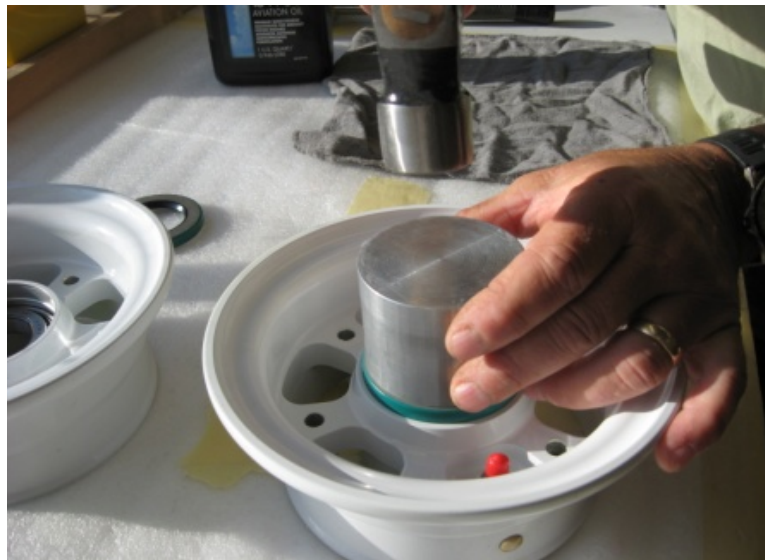
FIGURE 32-40-10-02-c Seat the grease seal with a hammer or a Press, using a properly sized drift, suitable to fit inside the wheel hub, but closely sized to the seal outside diameter.
