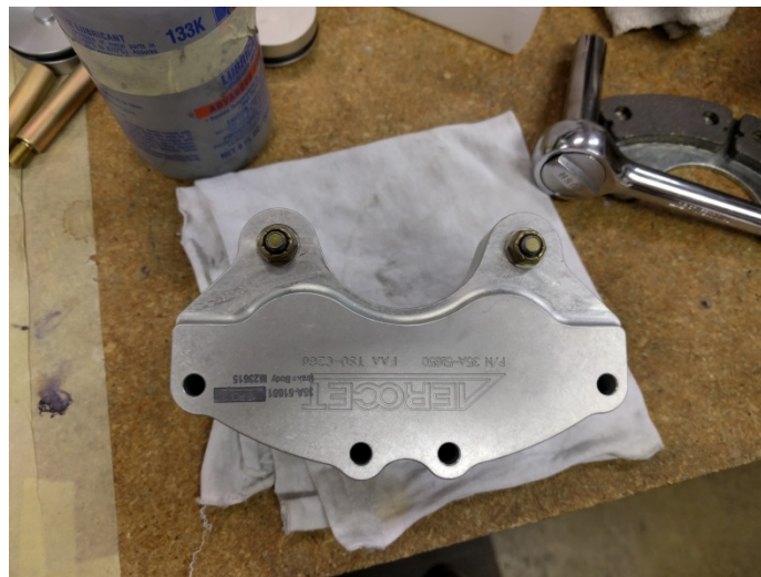
FIGURE 32-40-10-04-f Bolting anchor pin bolts.
