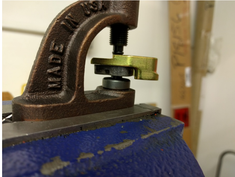
FIGURE 32-40-10-04-c Riveting Brake lining to back plate.
