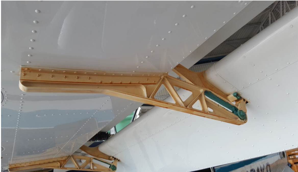
Plate 7: Flap Tracks Sprayed with AV-30
