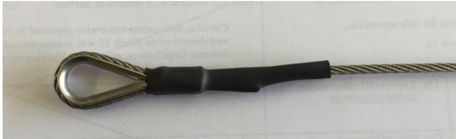
Figure 15-10: Insulation Sleeve over Nicopress
