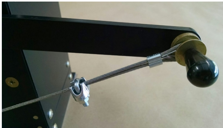
Figure 15-9: Securing Temporary Position with U-Bolt Clamp
