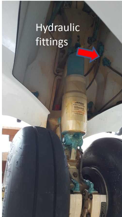
Plate 9: Landing Gear and Hydraulic Fittings with AquaShield™ and ARDROX AV 30
